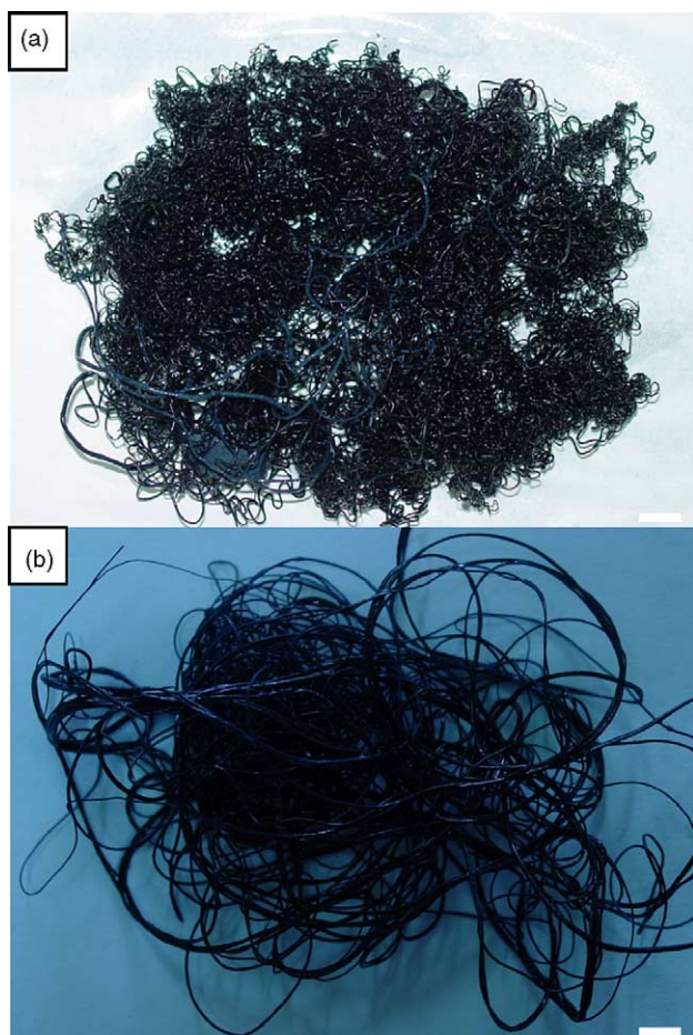
Fig. 2. Digital photographs of as-spun single fibers from (a) MWNT- g-p PEK and (b) VGCNF- g-p PEK in PPA/P 2 O 5 dopes. Scales bars are 1 cm.
